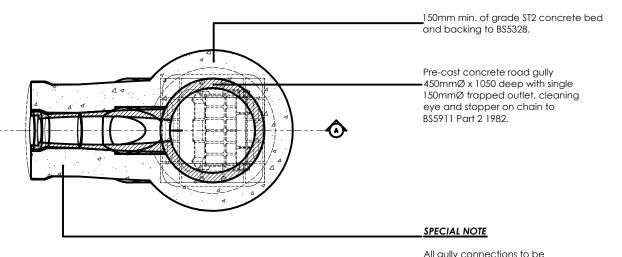
All gully connections to be bedded and surrounded in 150mm thick grade ST2 concrete for entire length irrespective of depth.
