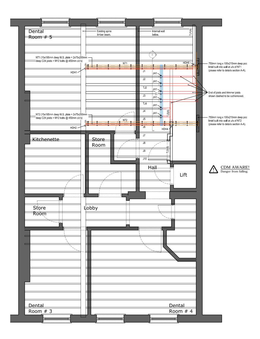
Second Floor Plan (showing structure above) - alterations Stage 2
